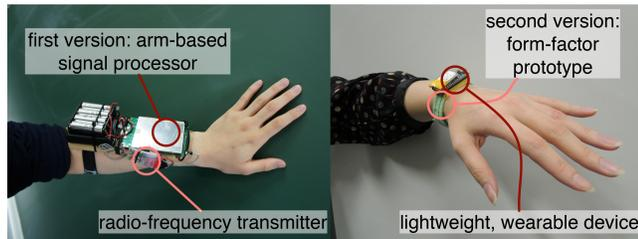
**Figure 1:** Two iterations of i-me TOUCH, showing the shrinking form-factor.
